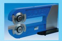
Manual machine suitable to separate pre-assembled Electronic Board. Precise, reliable and safe. The PCB is manually fed between the lower and upper blades using the scoring as reference. By pushing the board horizontally, the blade rotation starts offering a sharp and accurate cut. The blade height is adjustable depending on the thickness of the PCB. Upper and lower blades are also available titanium pleated version
