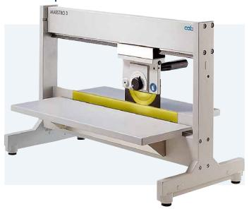
The MAESTRO 3E separates both small and large PCBs. The support table and the rest can be set continuously to the best possible operational position. By adjusting the distance between the linear blade and the rest, margin strips can fall through and are sorted out.
